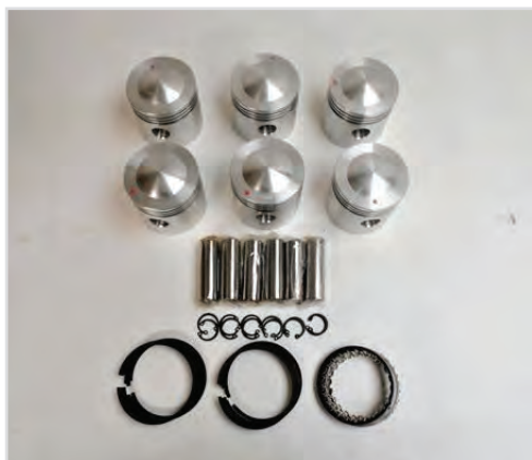
Dome top pistons fitted from engine KE10000
