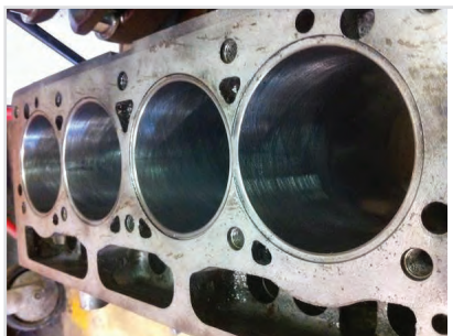
Engine block with recesses used for the later dome top piston engine after engine number KE10000
